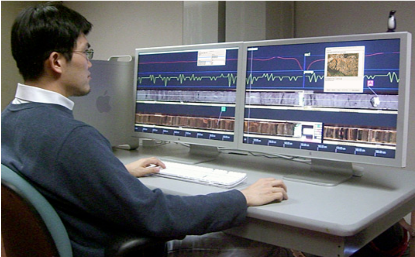
Julian Yu-Chung Chen in front of two 30" Apple Cinema Displays and a MacPro running Corelyzer, displaying high resolution core image along with sensor data plots.
